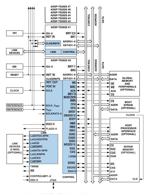
Figure 4. ADSP-TS202S Shared Memory Multiprocessing System
