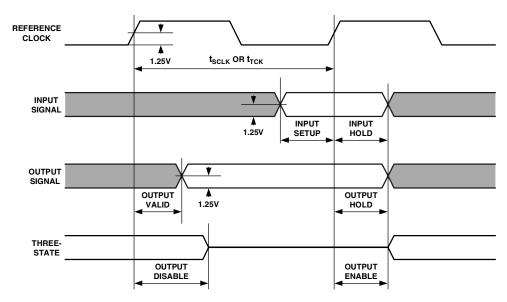
Figure 15. General AC Parameters Timing
