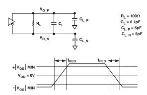
Figure 19. Link Ports—Differential Output Signals Transition Time
