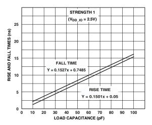
Figure 38. Typical Output Rise and Fall Time (10% to 90%,  $V_{DD\_JO}$  = 2.5 V) vs. Load Capacitance at Strength 1
