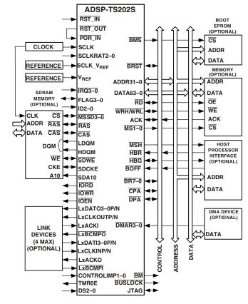
Figure 2. ADSP-TS202S Single-Processor System with External SDRAM
