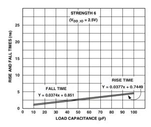
Figure 43. Typical Output Rise and Fall Time (10% to 90%,  $V_{DD\_JO}$  = 2.5 V) vs. Load Capacitance at Strength 6
