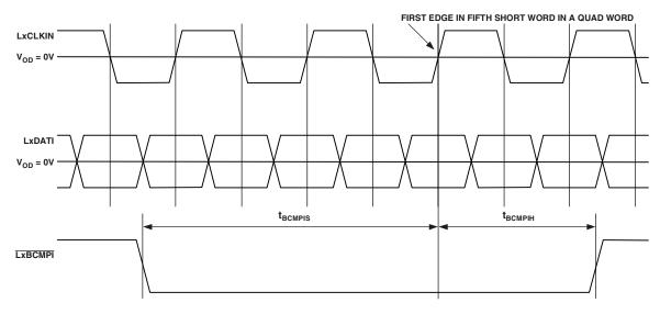
Figure 24. Link Ports—Last Received Quad Word
