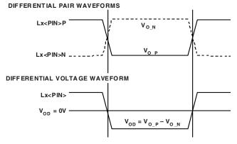
Figure 17. Link Ports—Signals Definition
