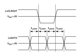
Figure 20. Link Ports—Data Output Setup and Hold<sup>1</sup>
