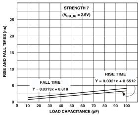
Figure 44. Typical Output Rise and Fall Time (10% to 90%,  $V_{DD\_IO}$  = 2.5 V) vs. Load Capacitance at Strength 7
