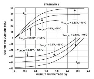
Figure 29. Typical Drive Currents at Strength 3
