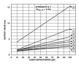
Figure 45. Typical Output Valid ( $V_{DD\_IO} = 2.5 \text{ V}$ ) vs. Load Capacitance at Max Case Temperature and Strength 0 to  $7^1$
