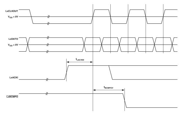
Figure 21. Link Ports—Transmission Start
