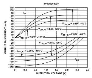
Figure 33. Typical Drive Currents at Strength 7
