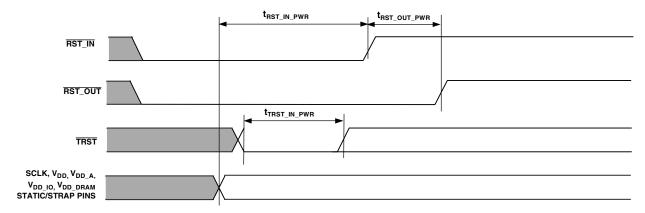
Figure 13. Power-Up Reset Timing
