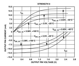
Figure 26. Typical Drive Currents at Strength 0
