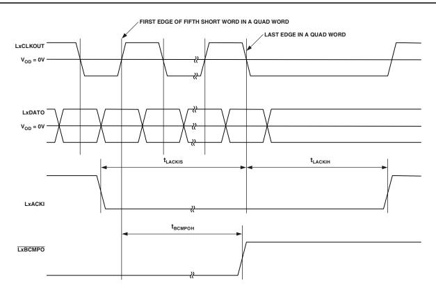
Figure 22. Link Ports—Transmission End and Stops
