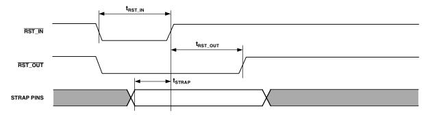
Figure 14. Normal Reset Timing
