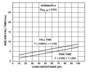
Figure 40. Typical Output Rise and Fall Time (10% to 90%,  $V_{DD\_JO}$  = 2.5 V) vs. Load Capacitance at Strength 3
