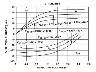
Figure 28. Typical Drive Currents at Strength 2
