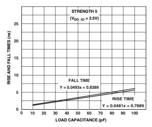
Figure 42. Typical Output Rise and Fall Time (10% to 90%,  $V_{\rm DD\_IO}$  = 2.5 V) vs. Load Capacitance at Strength 5
