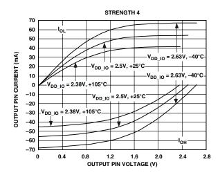
Figure 30. Typical Drive Currents at Strength 4
