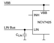
Figure 2. Master with Pull-up to VBB
