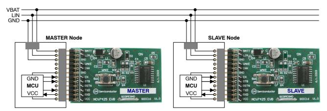
Figure 5. NCV7425 Evaluation Setup Connection
