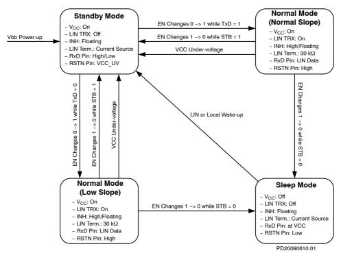
Figure 6. NCV7425 State Diagram
