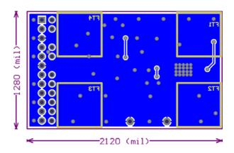
Figure 11. NCV7425EVB PCB Bottom Composite Drawing (Mirrored)
