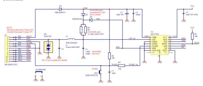
Figure 7. NCV7425 LIN Transceiver with Voltage Regulator and Reset Pin Evaluation Board Schematic
