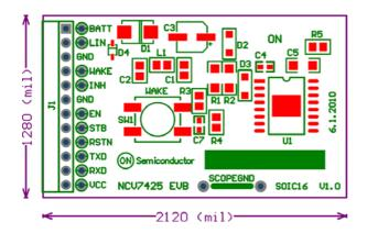
Figure 8. NCV7425EVB PCB Top Assembly Drawing
