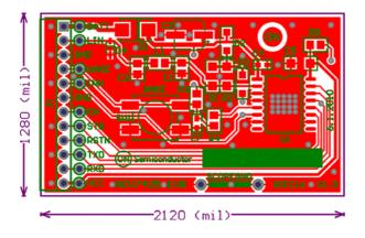
Figure 10. NCV7425EVB PCB Top Composite Drawing
