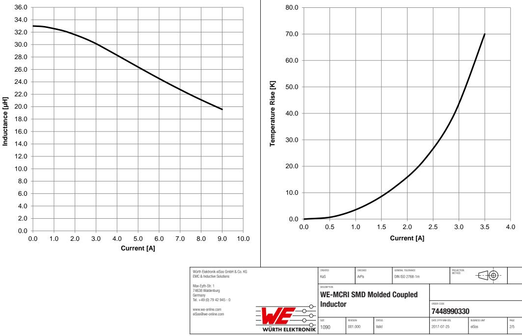
**Typical Temperature Rise vs. Current Characteristics:**
