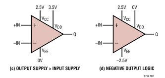
Figure 2. Typical Power Supply Configurations (Applicable to the LTC6752-2/LTC6752-3/LTC6752-4)
