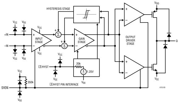
Figure 1. LTC6752/LTC6752-1/LTC6752-2/LTC6752-4 Block Diagram
