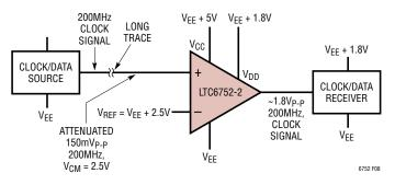
Figure 8. High Speed Clock Restoration/Level Translation/Level Shifting Circuit
