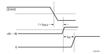
Figure 7c. Input State Not Held Long Enough. Wrong Output State Latched
