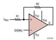
Figure 6. Additional Hysteresis Using Positive Feedback
