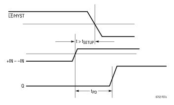
Figure 7a. Input State Change Properly Latched
