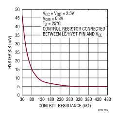
Figure 5. Hysteresis vs Control Resistor
