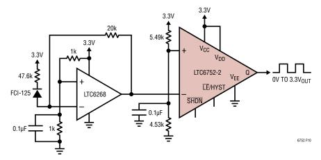
Figure 10. Optical Receiver Circuit
