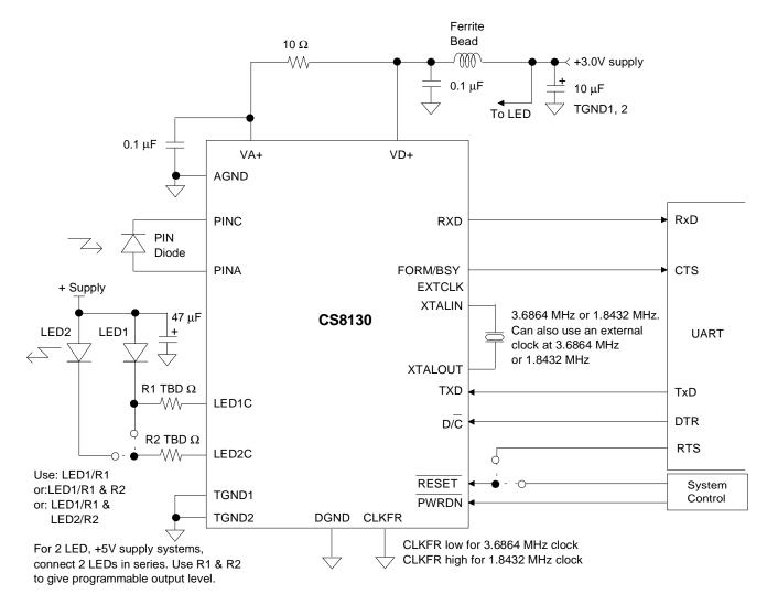
Figure 1. Recommended Connection Diagram
