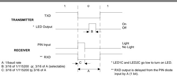
Figure 2. Infra Red Data Format Mode 1 (IRDA/HPSIR)
