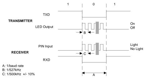
Figure 3. Infra Red Data Format Mode 2 (500kHz ASK)
