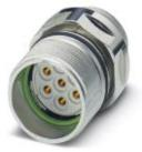
Device connector for front wall, straight, shielded: yes, SPEEDCON locking, M23, No. of pos.: 8+1, type of contact: Socket, Crimp connection, Axial seal, Central fastening M20 x 1.5, can be positioned via a locking nut
