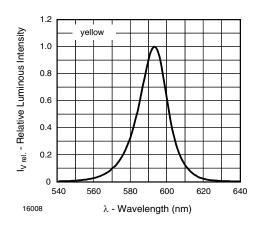
Fig. 3 - Relative Intensity vs. Wavelength
