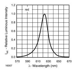
Fig. 2 - Relative Intensity vs. Wavelength
