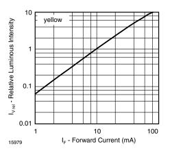
Fig. 6 - Relative Luminous Flux vs. Forward Current
