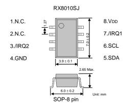
The metal case inside of the molding compound may be exposed on the top or bottom of this product. This purely cosmetic and does not have any effect on quality, reliability or electrical specs.
