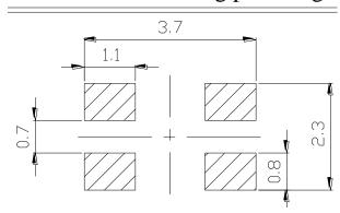
Note: Tolerances unless mentioned ±0.1mm. Unit = mm
